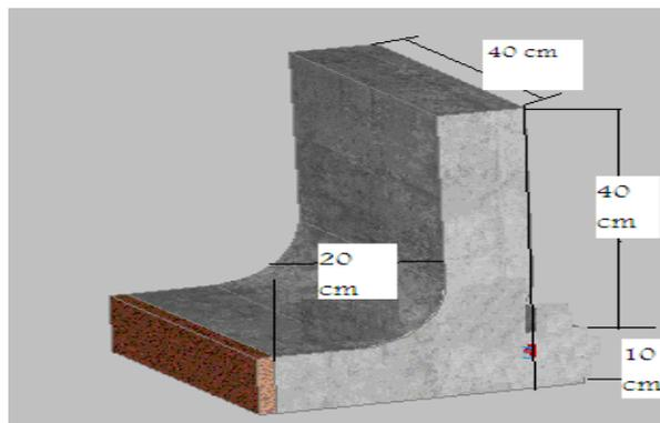
**Fig. 1. Dimensions of a precast unit**
